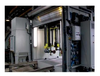
Whether testing or painting measures – the basis for any form of processing of demounted wheelsets is their comprehensive cleaning from dirt, rust or old paint. The cleaning plant conceptualized for this is equipped with brushing- and grinding tools and works completely automatically. According to the respective specifications wheelset shafts can be dry-cleaned at complete wheelsets or individually.
