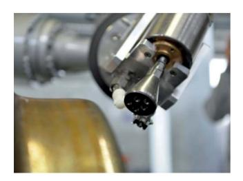
By this system, railway wheelsets and bogies for subsequent processes using the high-pressure water blast method robot-supported cleaned or de-coated, without causing changes to the surfaces, as occurs by abrasive methods.
