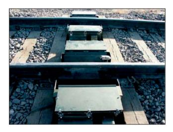
The stationary measuring device is used to measure different parameters on mounted wheelsets during the passing over of the device with self-driving of the trains. The device is primary installed on journey paths in the enter area of workshops / depots. The condition of the wheelsets are continuously monitored and preventive measures for necessary repairs can be derive.
