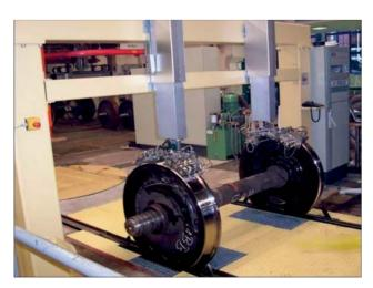
The in use internationally proven plant make it possible to check wheel discs full-automatically for cracks in the structure for other stress injuries.
