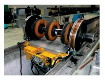
The in the track area mobile ultrasonic testing device enables to test automatically all wheelsets under mounted state on the stationary train. In accordance to the general state testing requirements will be the results displayed or stored. From the testing of individual areas, such as outer running surface or rim, longitudinal, transverse and volume error can be detected and the forthcoming maintenance arrangements can be defined.
